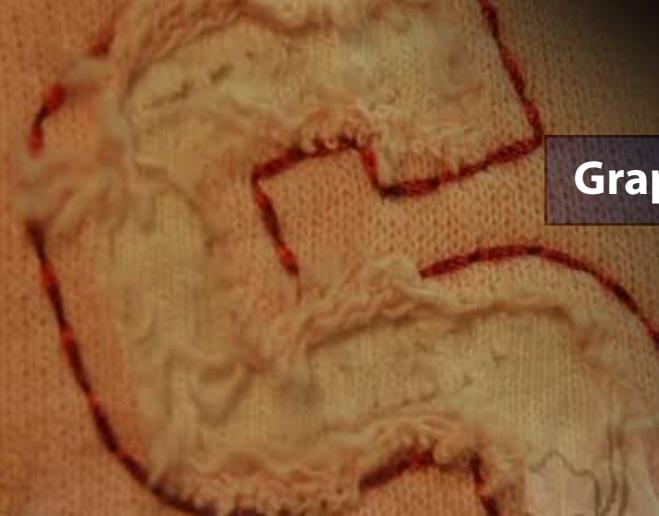
🇬🇧 As well as being able to cut appliques for embroidery, the Graphixscan can control its power so precisely, it is able to cut only through one layer of fabric leaving the material underneath untouched., this allows for the creation of pre stitched appliques to be cut whilst still in the embroidery frame. Simply attach your existing embroidery frame carrier to the cutting bed and you will have perfect registration every time.
